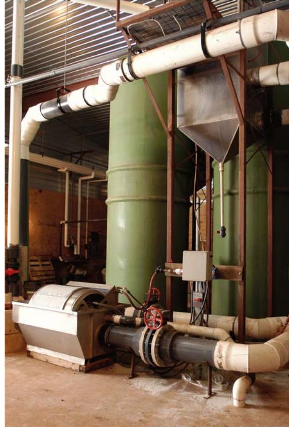
**Figure 5. The two green columns are biofilters. Note the degassing/LHO unit at the top of the biofilter on the right.**
