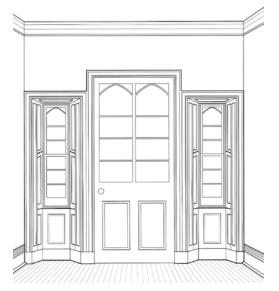
A transom window was often installed above the door to let light and air into the entry on the other side. If the entry hall was wide enough, the door could also feature sidelights on either side.
