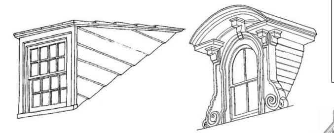
**Adding a dormer** – If you want to add a dormer, do so in keeping with the style of the house. Consult with an expert before cutting into the roof of your house. A window installed in the gable end or a skylight installed less obtrusively on the rear elevation may be the solution to improving the light and ventilation of an attic space.
