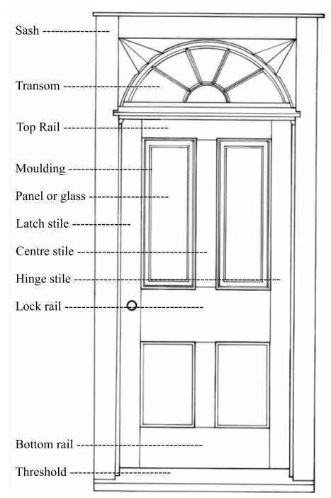
When replacing a door, give some serious thought to having a millwork or woodworking shop build an exact duplicate. It's doubtful that you'll be able to find a new door that exactly fits your existing sash. Installing a factory-built door will, in most cases, mean demolishing existing sash, which in turn means removing and repairing trim and mouldings and, in many cases, exterior sheathing and interior wall finish. A custom-built door can be hung in the existing sash.
