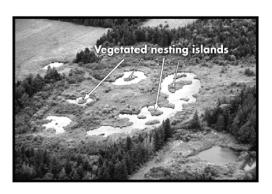
Sites for wetland enhancement ponds should be chosen with soils capable of retaining water in order to maintain an adequate water depth throughout the nesting season. A suitable water depth, typically 50 to 100 centimetres (0.5 to 1 metre), is important to establish vegetation and aquatic organism populations.
