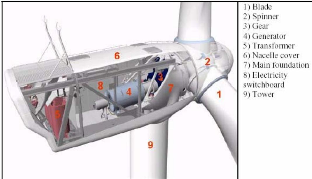
Figure 3.2.Components of the V90 nacelle (Vestas, 2005)
